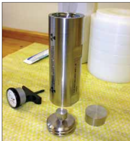
Special form capsules had to be used to guarantee PUBE and AMBE containment, even under extreme conditions.
