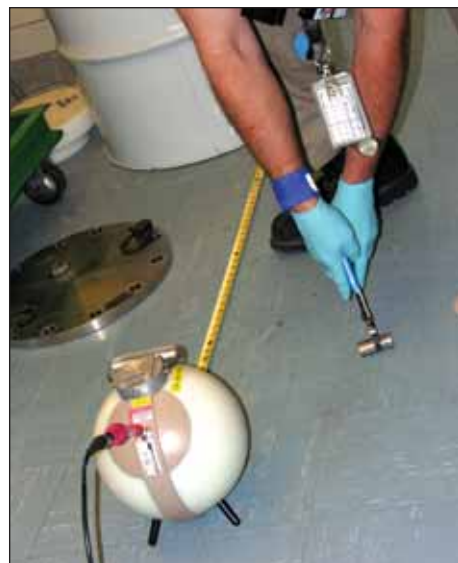
Neutron measurement of the PUBE source
