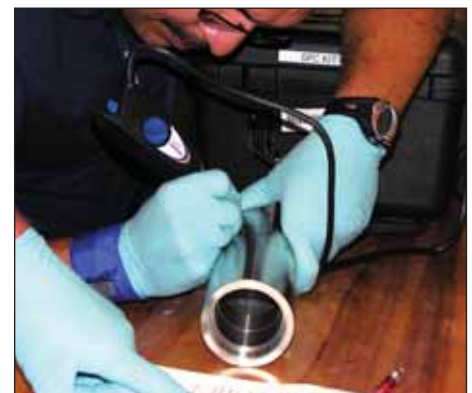
Special form capsules had to be used to guarantee PUBE and AMBE containment, even under extreme conditions.
