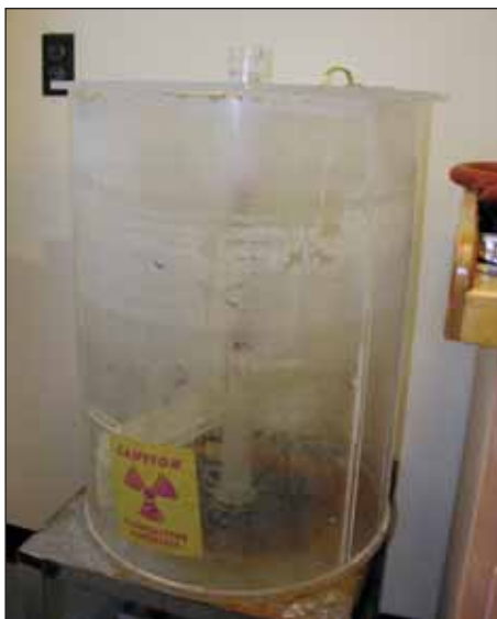
Visiflux II Neutron Howitzer apparatus containing the PUBE source
