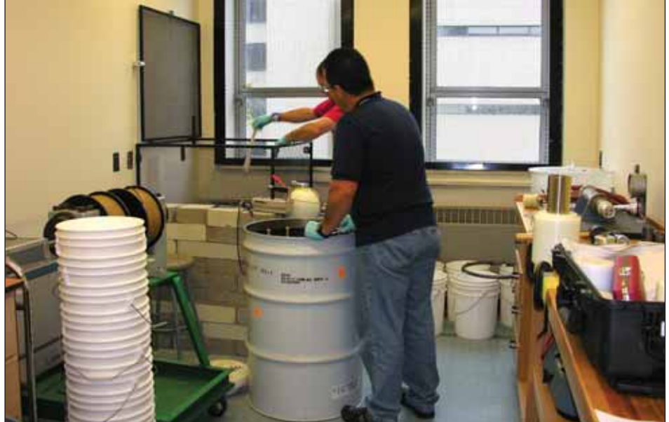
Removing the PUBE from the Neutron Howitzer, concrete blocks act as a shield against neutron exposure
