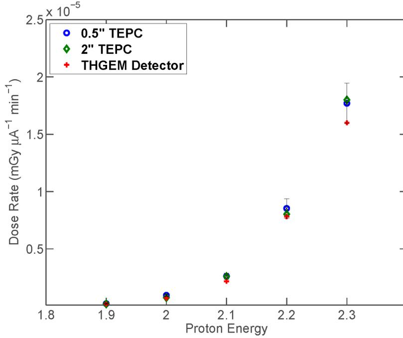
Figure 6: Measured dose rates obtained from the prototype multi-element THGEM detector, 0.5 and 2 inch standard TEPCs at different proton energies.
