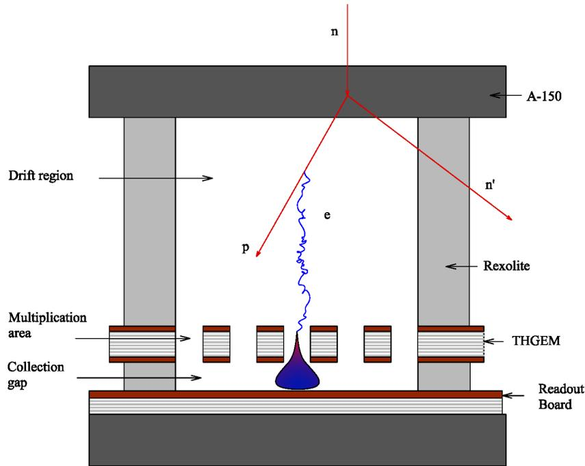
Figure 1: Schematic view of different functional gas areas in a single gas cavity of the prototype THGEM-based detector.
