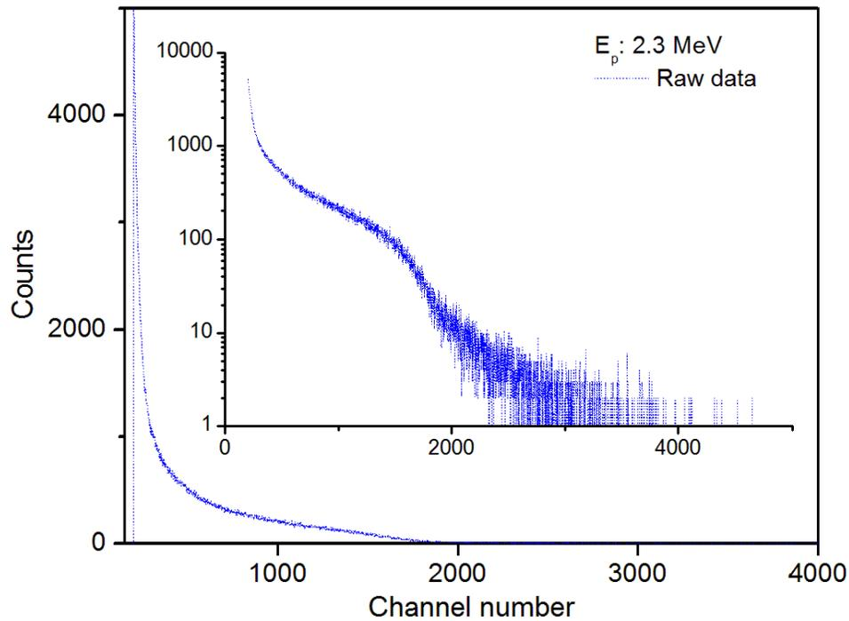
Figure 4: The pulse height spectrum obtained using the prototype multi-element THGEM detector at a THGEM bias voltage of 650 V and for a proton energy of 2.3 MeV.
