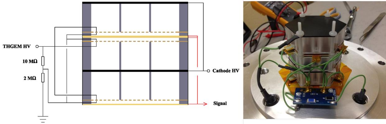
Figure 2: A schematic diagram of the bias voltage connections and a photograph of the multi-element THGEM detector within the aluminum casing.
