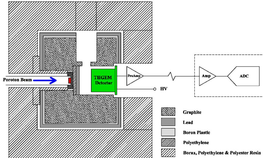
Figure 3: The arrangement of the measurement setup with THGEM detector.
