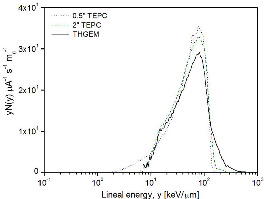
Figure 5: The lineal energy spectra obtained using the prototype multi-element THGEM detector and commercial TEPCs after gamma-ray component elimination.
