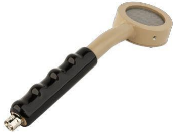
thin window GM "pancake" - \alpha\beta\gamma
