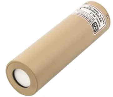
thin NaI - \uparrow energy \beta , \downarrow energy \gamma
