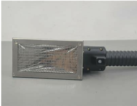
thin ZnS sandwiched to plastic scintillator "dual phosphor" - \alpha/\beta\gamma
